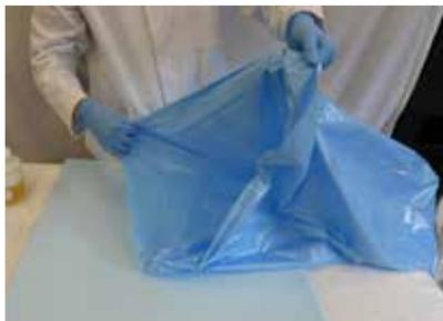
Place the bag onto a piece of wood or foam board for best foam rise. Snap open bag, fold evenly from each side, folding underneath.
