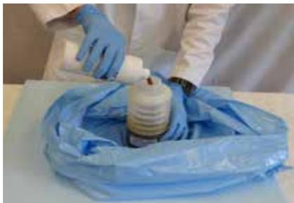
Place bottles in bag for safety. Remove caps, expand bottle #2 and pour entire contents of bottle #1 into #2.
